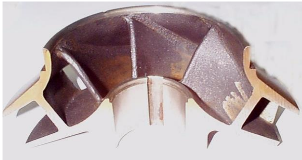
Figure 4 Sectioning of the Impeller
