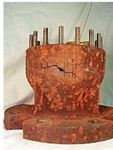
Figure 2 Corroded/Cracked Pump Bowl
