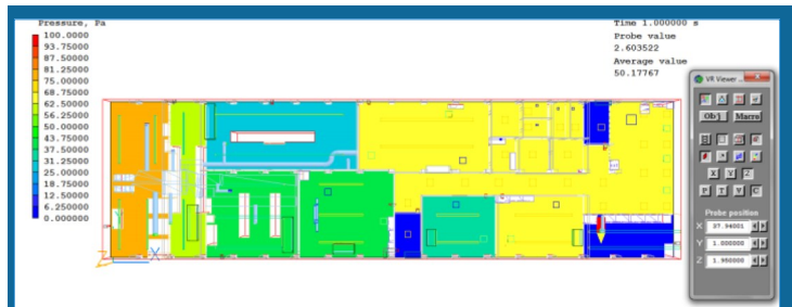
Fig 8: Plot of Pressure Ranges in Rooms after 1 sec., in emergency mode—Scenario 3
