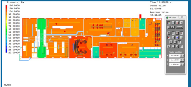
Fig 4: Plot of Pressure Ranges in Rooms after 11 sec., in summer mode—Scenario 1
